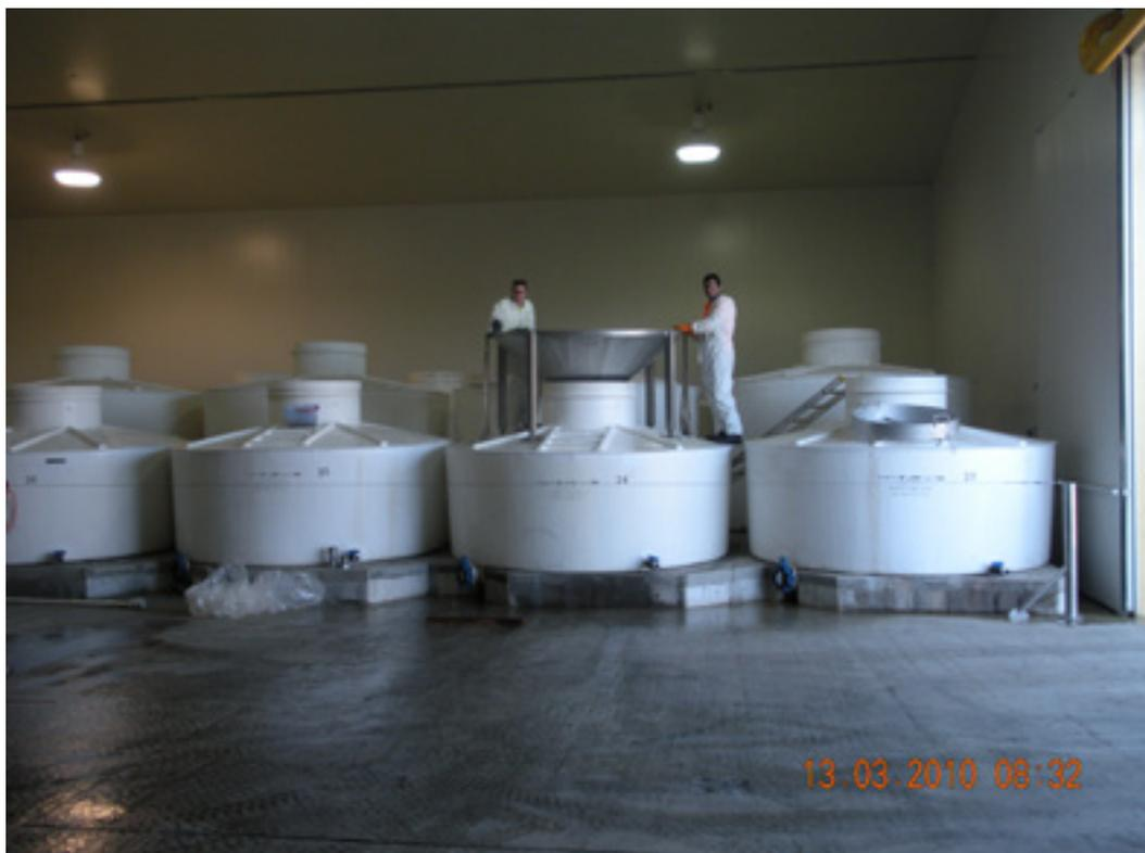
**Figure 6: Safety-clad operators ready to control lye-treated olives being tipped into a processing tank**
